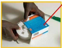
If you have a smoke alarm with a 9-volt battery, replace the battery **EVERY YEAR**
